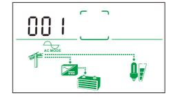
2) AC input interface(Display AC input voltage and frequency)
