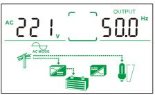
3) Battery interface(Display battery voltage and percentage)
