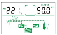
3)Battery working mode (No mains input)
